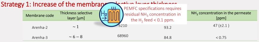
Reaction temperature = 500 C, reaction pressure = 4 bar(a), ammonia feed flow rate =  $0.5 L_N/min$ .
