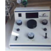
Elium pycnometer (Model 1305 Multivolume, Micromeritics)
