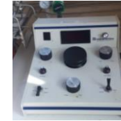
Elium pycnometer (Model I305 Multivolume, Micromeritics)
