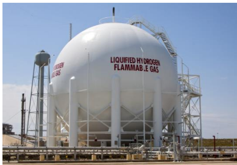
Figure 12: Liquid Hydrogen Storage Spheric Tank. Source: NASA.
