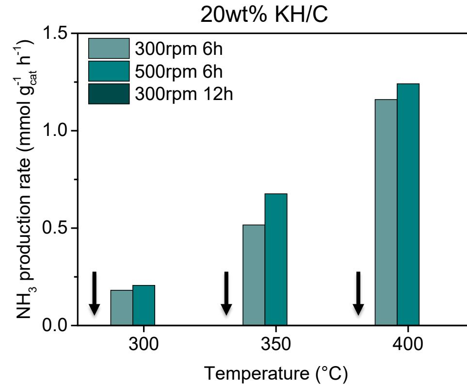
BM can be used to synthesize KHC ammonia catalyst, but prone to destruction
